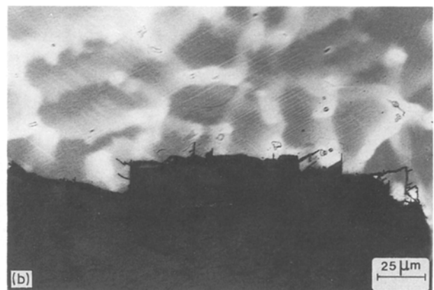
Figure 5 Optical micrographs of the side views of the fatigue fracture surfaces showing the effects of nickel additions on the fatigue crack propagation mechanism, (a) alloy 1 and (b) alloy 3.
