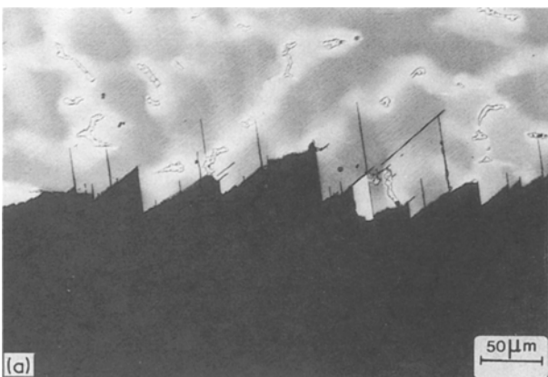
Figure 5 Optical micrographs of the side views of the fatigue fracture surfaces showing the effects of nickel additions on the fatigue crack propagation mechanism, (a) alloy 1 and (b) alloy 3.
